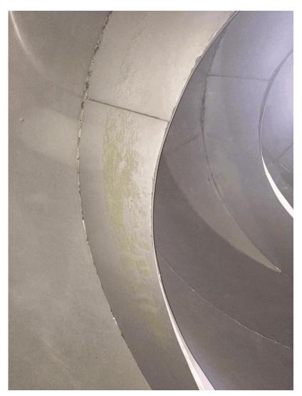
An internal photo of one of their mixer drums which had been using the DrumBlaster for 4 months was also given to us showing no build up at all.
